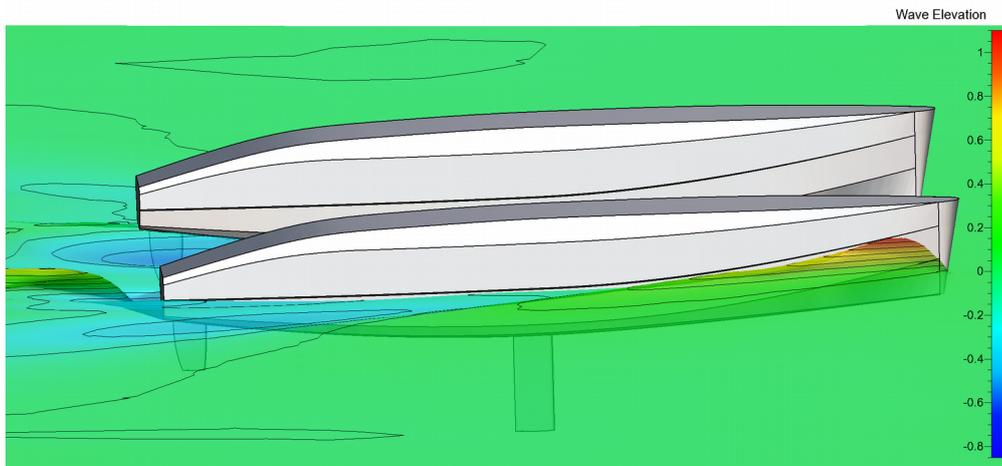
Wave elevation: Clean run-off at the submerged hull
