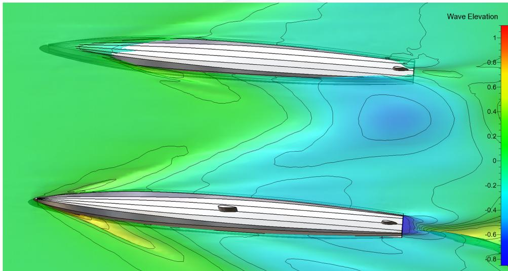
Wave elevation: Bottom view, no rudder ventilation
